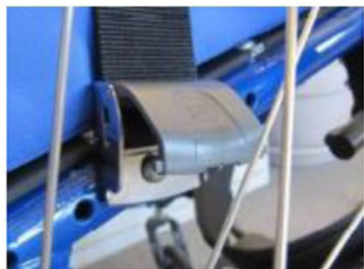
Figure 6. Locking clamp end-fitting webbing adjustment
