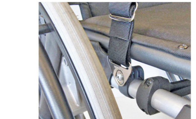
Figure 4. Triangular end-fitting and three bar slide webbing adjustment
